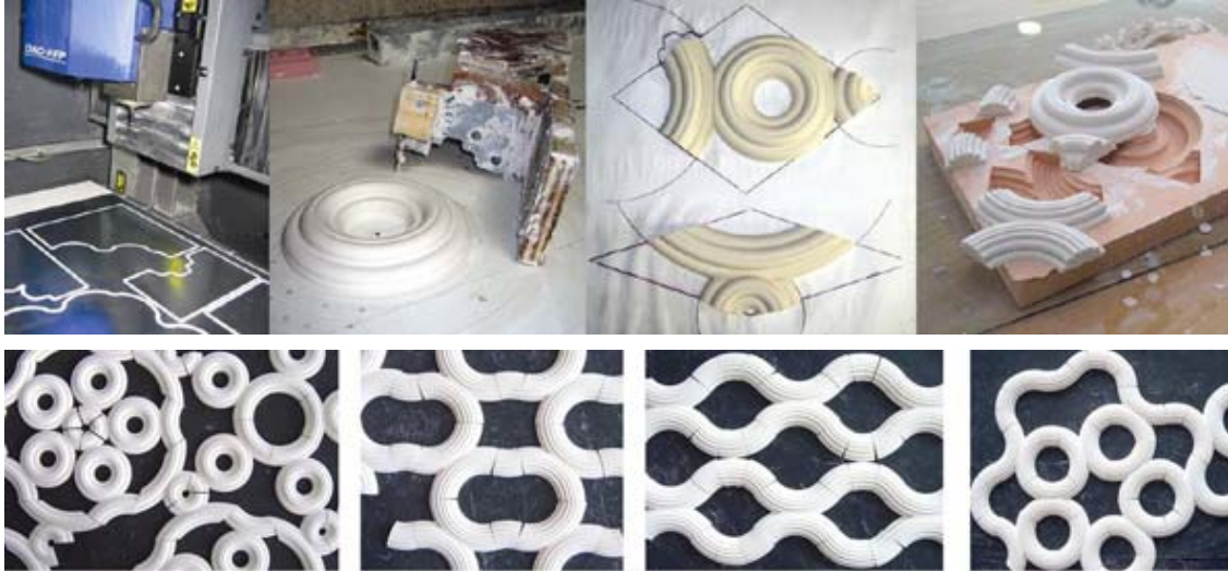
Fig 8 CNC milling of metal profiles, spinning of plaster, construction of master models, moulded test units.
