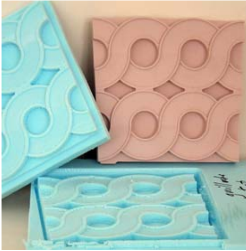
Fig 3 CNC milled 'guilloche', foam tests and final milled master 300x300x20mm approx.
