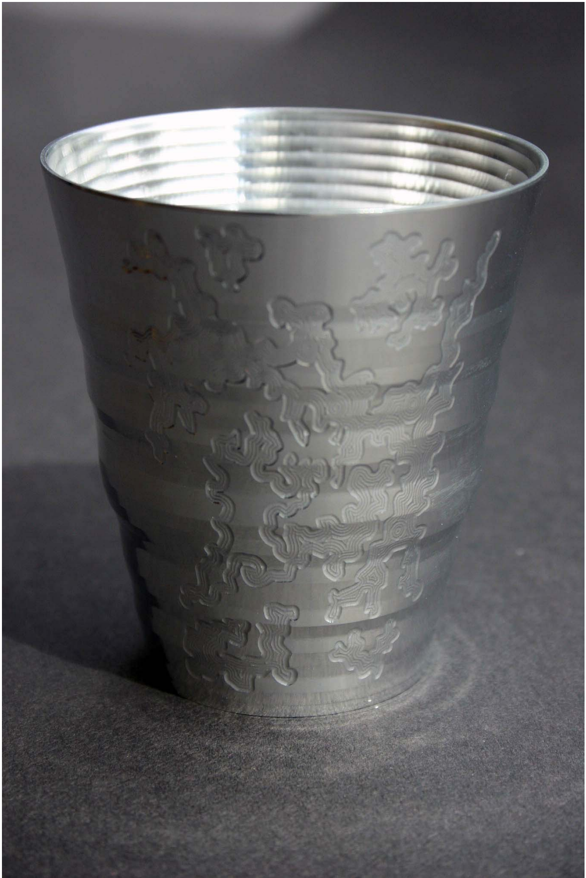
Figure 15: 'Whisky Tumbler', 4 axis CNC milled Aluminium, 80mm diameter, 80 mm depth. The Pattern is a consistent depth despite the undulating surface.
