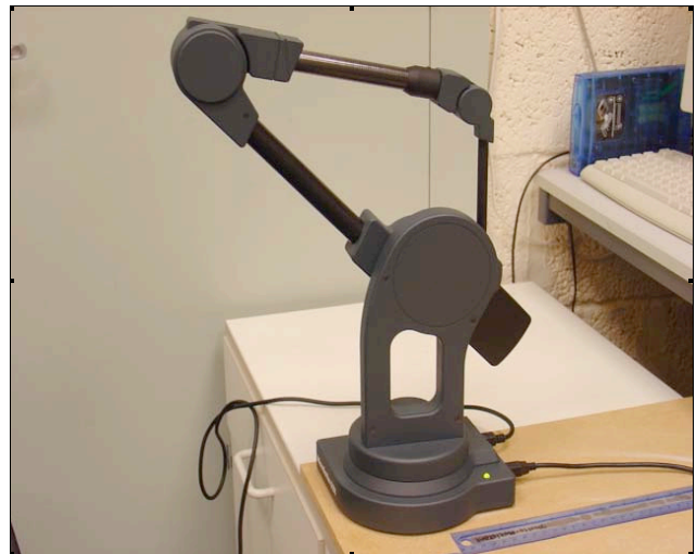
Fig 3. The G2 Microscribe digitising arm from Immersion Inc.
